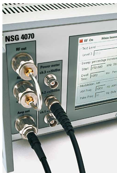
NSG 4070 front panel with RF ports
